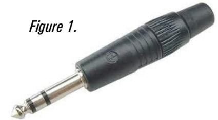
Figure 1. A TRS connector with the three conductors separated by the black insulation bands. The pointed front of the connector is the tip, the middle band is the ring, and the large conductor at the rear nearest the plug body is the sleeve.
