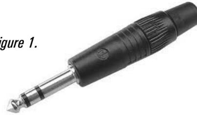
Figure 1. shows a TRS connector with the three conductors separated by the black insulation bands. The pointed front of the connector is the tip, the middle band is the ring, and the large conductor at the rear nearest the plug body is the sleeve.
