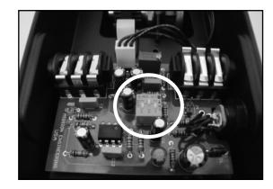
SW1: Active/Passive switch. Default ON (passive). This switch should be left on for most passive (un-powered) guitar pick-ups. If using active, or very hot pickups, the internal amplifier in the VM-PRO™ may be driven into distortion. If this occurs, set SW1 to OFF for active pickups.
